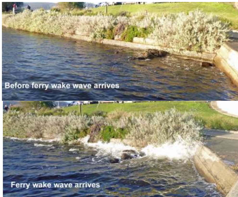
Figure 7: Commuter ferry boat wake viewed from the Kangaroo Bay South shore at photo point KBPP4 (see below and Appendix 1) close to high tide during calm weather on 17 th August 2021. The ferry (not visible) was about 170 metres offshore, travelling eastwards into Kangaroo Bay and slowing down at the end of its river crossing. Top: Calm water before boat wake arrival. Bottom: Boat wake wave arrives at shore, a few seconds after top photo.
