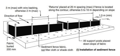
4. Sediment fences. Install parallel to the contour with ends angled upwards. Bury fabric 200 mm deep, Join sections of fabric at a support post with a 2 m overlap. Ensure fabric is securely attached to all support posts. Not suitable for concentrated flow paths, creeks, or major drainage lines.
