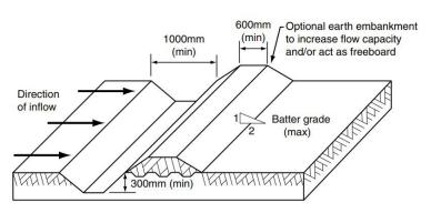
1. Diversion drain. The drain channel must be at least 150 mm deep with a curved shape that will be site specific. Stabilise the flow path to protect it from scour by lining the drain with matting or rock. If dispersive soils are present, create diversion drains by building soil berms instead of diagina.
