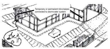
**2. Early drainage connection.** Connect downpipes and other drainage to the stormwater system as soon as the roof is on and / or other impervious surfaces are constructed, such as driveways, parking areas, or the building slab. Temporary flexible downpipes can be useful until permanent pipes and drainage system is in
