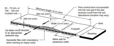
3. Stabilised site access. Stabilised access is from the site boundary to a formal stockpile area or work site; minimum length for small developments is 10 m. Strip at least 150 mm of topsoil, cover with geotextile then a 200 mm thick pad. Divert water from this control to appropriate sediment controls.
