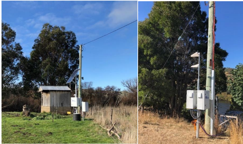
Figure 1a: Installation examples of Eco Detection units. Left: Ouse, device mounted on a pole with solar power. Right: Derwent below Meadowbank dam, device mounted with ground screw and pole, access to mains power, and antenna.
